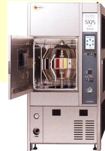
xenon-arc lamp artificial weathering
