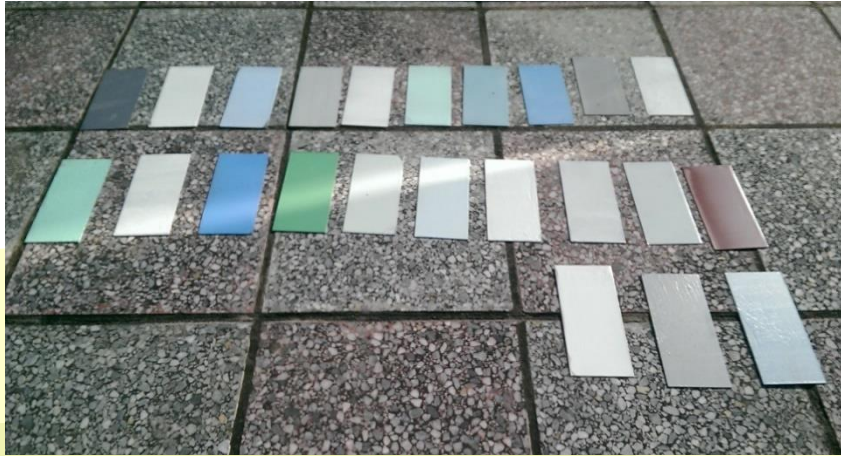
Natural weathering (steel substrates)
