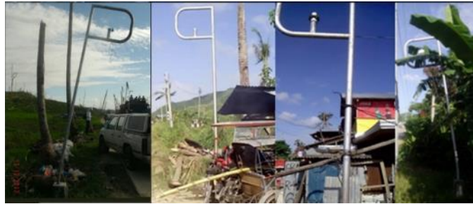
Figure 8: Windicators (L to R: #4, #10, #9 and #8) These were lamp posts installed in 2010 at Palo, Leyte. Windicator #9 was included in the study for verifications whether it was tampered or not.
