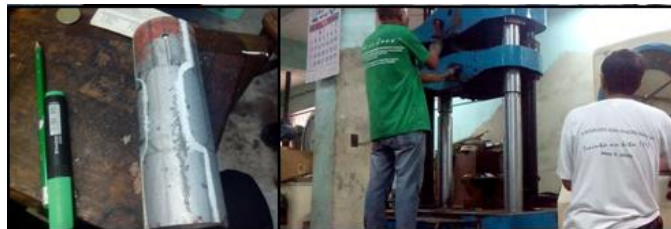
Figure 9: Tensile test (right) on the sample (left)
