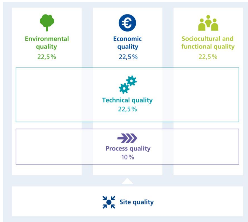
Figure 1: The basic DGNB evaluation structure
