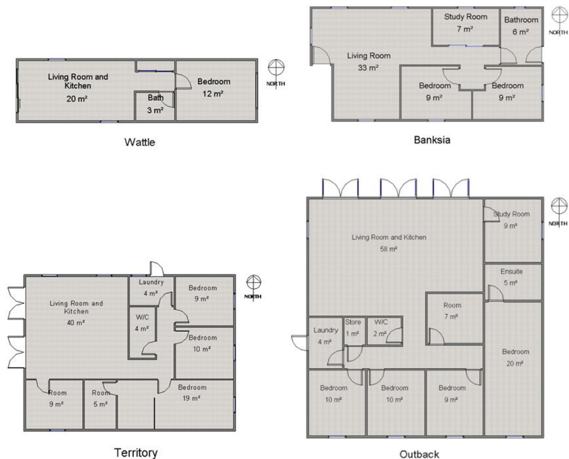
Figure 1: Floor plans of the four sample buildings
