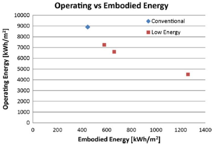
Figure: Operational and embodied energy for case studies (Source: Ramesh et al., 2010)
