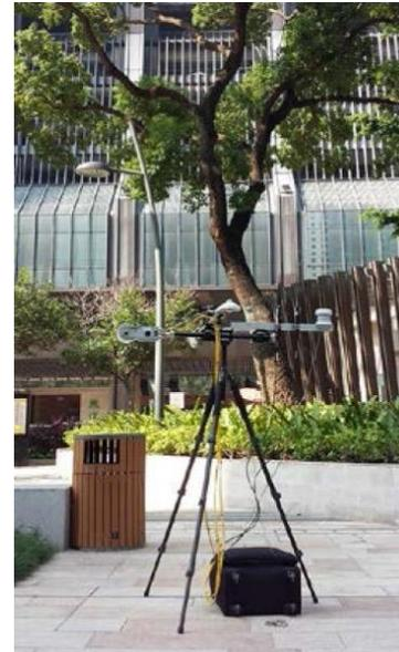
measure Short-wave and long-wave radiation
