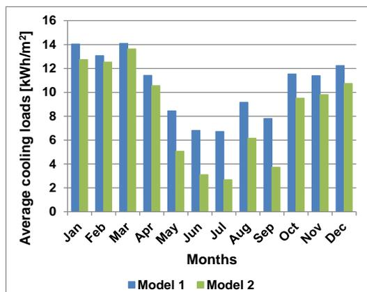
Figure 3 – Comparison of cooling loads of DSF models 1 (fully air conditioned) and 2 (mixed mode ventilation)
